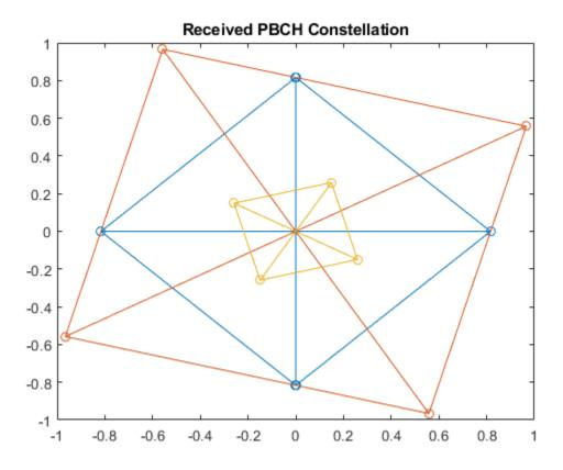
Equalize the symbols by performing MMSE equalization on the extracted resources. Plot the results.
